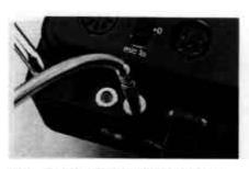
You can use a wire manual release to manually shoot single frames or, to start and stop the camers with the swivelling lever of the tripod.
