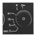
You must cut out the programming by turning switch 31 from the «red dot» marking to • ■ 1» and then back to the «red dot». LED 20 will then be extinguished.
