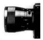
You can also shoot films without exact range metering by adjusting the camera to its \*snapshot setting\* or red dot setting.
