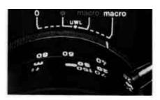
When filming with the power zoom, turn the knurled ring with the white mark to the red marking "macro". Sight the object. Then precisely focus the camera with the rocker button 4 for the power zoom.
