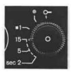
The automatic single-frame system permits effective time-lapse shots. However, you must have a very solid tripod. The best idea is to screw your camera onto a three legged tripod and to set switch 26 to 18 or 16 2/3. Set switch 31 to 15 s. A frame will then be exposed approximately every 15 s. This corresponds to a 270-fold time-lapse.
