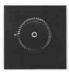
You can switch from the normal 18 fps filming speed or from 16 2/3 fps to single-frame operation, very easily.
