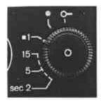
You can also shoot single frames manually with a wire release or with the Nizo remote release. You then have the filming speed and time-lapse effect at your control.
