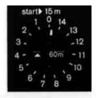
You can read off the available film footage in meters by means of the footage indicator 23.
