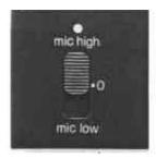
Shift the slide switch 39 to -mic high- (red dot marking).
