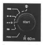
For pre-programmed and automatic fading-in and fading-out of the following scene, set switch 25 to the desired fade-in and fade-out
