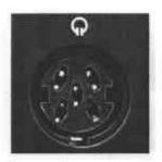
You can also connect commercially available headphones with an impedance of et least 1.5 kOhms to socket 40.
