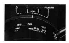
For filming with the ultra-wise lens, set the focusing ring to infinity ( $\infty$ ) and set the knurled ring 16 to the ~UWL~ marking with the white mark. Now, proceeding from the maximum zoom setting (56 mm or 80 mm) turn the zoom ring in the direction of ~mecro~ until it moves no further (manually or with the motor), thus achieving the exact UWL position. With this setting, and with the lens fully open, you have a depth of focus range from infinity ( $\infty$ ) to approximately 0.35 m.
