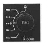
Before shooting a scene which you would like to begin with a fade-in, set switch 25 to the desired type of fade-in • ► • or • ► •. With the master switch 11 switched on, depress button 21. LEO 20 will then light up. Look into the viewfinder. Wait until the red area of the aperture scale is next to the index mark. Then carefully and briefly depress button 21 at the same time as you depress the release button 15. The following scene will then begin with the programmed fade-in.
