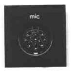
The microphone included has a directional characteristic and an impedance of 2000 Ohms. You can also use any other low or medium impedance microphone (200 to 5000) Ohms) which is wired in accordance with DIN 45 594. You will find a circuit diagram at the end of section four which will help you in your search for the right microphone.
