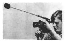
A microphone mounted on the camera is the best solution for one-man operation. However, in principle you should always try to place the microphone as near as possible to the sound source.
