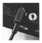
Insert the plug of the flash sync. into socket 43 of the camera.
