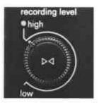
In most cases, you can leave the recording level control to the infinitely variable automatic system when using the microphone.
