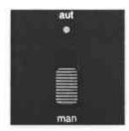
The automatic sound recording level system always sets itself to the loudest sound source. Weak noises only reach the proper recording level after a slight delay.
